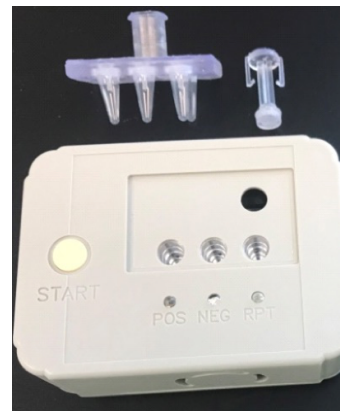
Prototype molecular diagnostic test platform for at-home use being developed in VIC Foundry. Disposable test cartridge and plunger (top) and reusable instrument (bottom).
