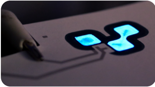
4-layer display printed with electroluminescent ink Read the white paper: voltera.io/EL
