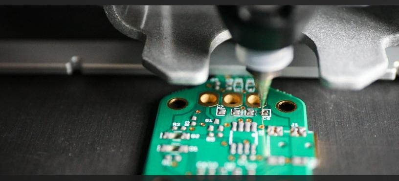
Along with printing custom circuit traces, the Voltera V-One can precisely dispense solder paste onto printed or factory-fabbed boards for rapid population of surface-mount components.
