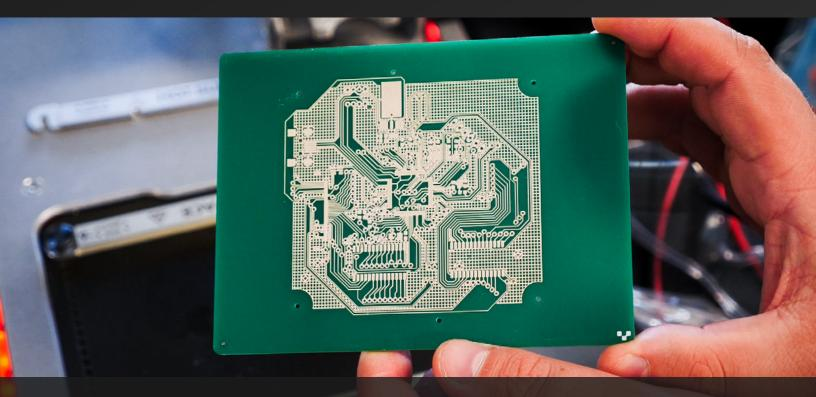
A 'graphical LCD and touchscreen overlay controller' printed and cured on an FR4 rigid substrate by the Voltera V-One.
