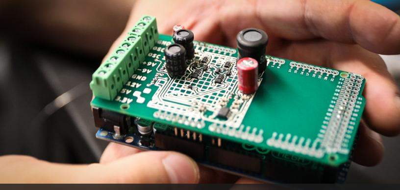
A 'switching power supply' printed on an Arduino Mega template shield. Custom traces, solder paste dispensing and reflow all accomplished on the Voltera V-One.
