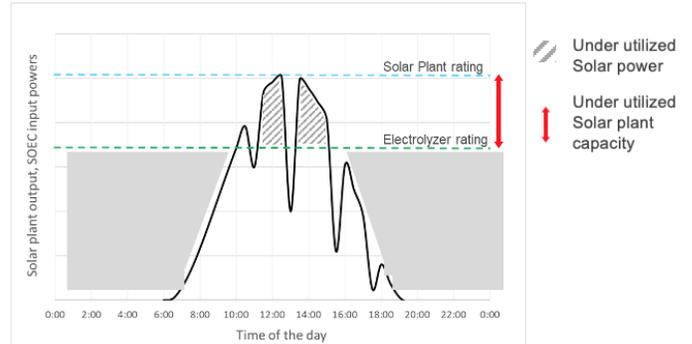
Deploying a combination of batteries and electrolyzers captures maximum energy and optimizes capital and operational costs (right). Both high and low temperature electrolyzers will benefit from this architecture, because both technologies will want to maximize the capacity factor of the equipment.
