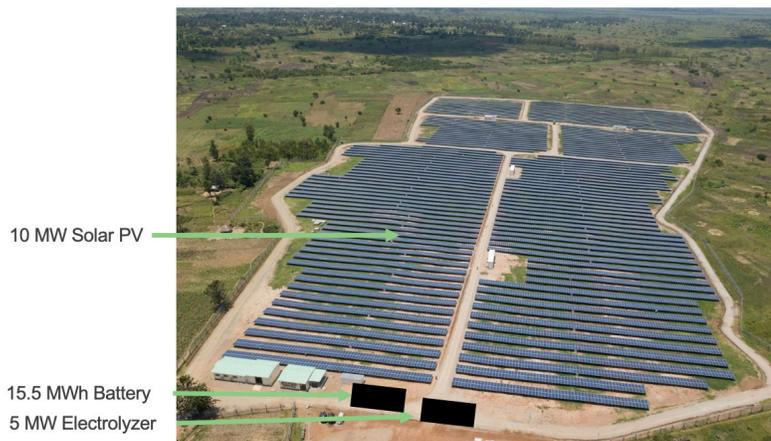
A small portion of this battery system can be used to keep high temperature electrolyzer stacks at their desired temperature when the renewable energy is not available.
