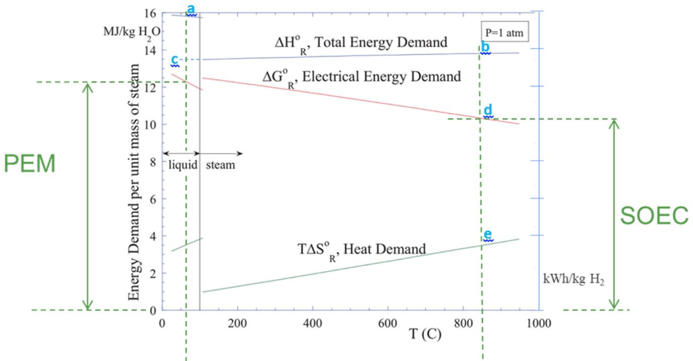
**FIGURE 1: ENERGY DEMAND AS A FUNCTION OF TEMPERATURE FOR ELECTROLYSIS OF WATER**
