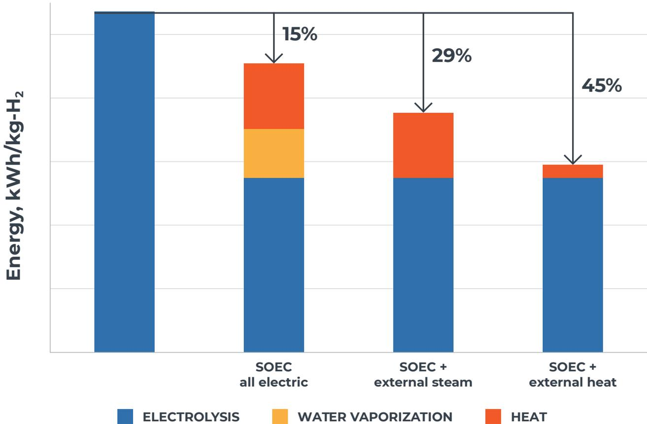
**FIGURE 2: ENERGY CONSUMPTION OF LOW TEMPERATURE AND HIGH TEMPERATURE ELECTROLYZERS**
