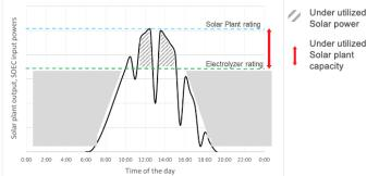
Deploying a combination of batteries and electrolyzers captures maximum energy and optimizes capital and operational costs (right). Both high and low temperature electrolyzers will benefit from this architecture, because both technologies will want to maximize the capacity factor of the equipment.
