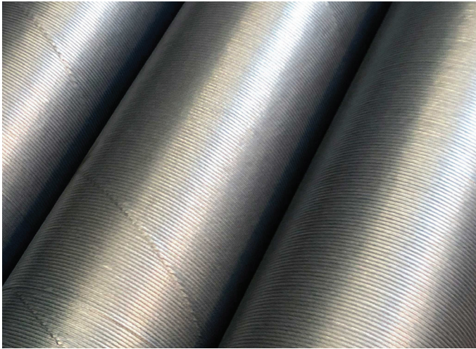
Refurbished Furnace Skid Posts Laser Clad in Colmonoy® 625
