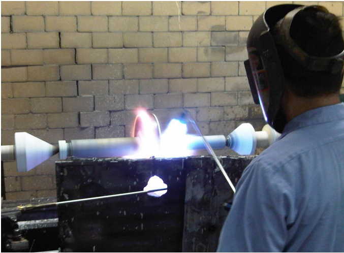
Fusing Colmonoy 52SA onto B.O.P. Ram
