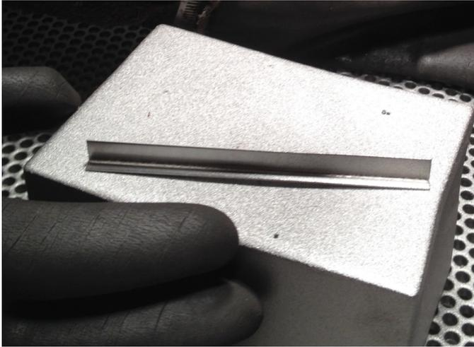
*NicroBlast Grit blasting process on T-Specimen.*
