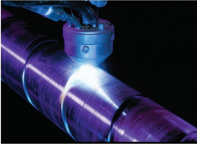
Wallex® 21 applied by PTA on Plastic / Rubber Industry Extruder
