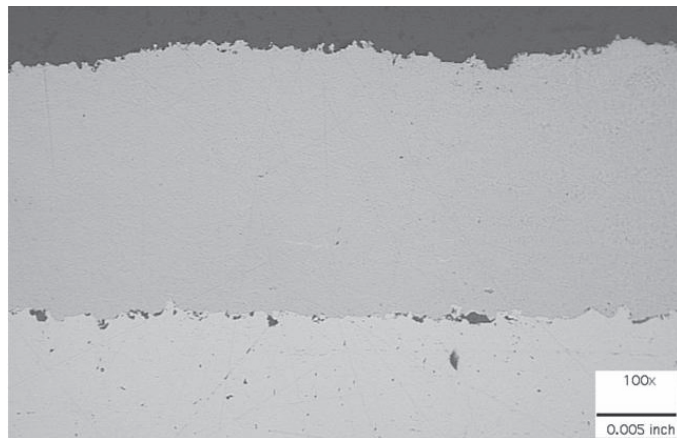
Photomicrograph of Colmonoy 88HV (original at 100x)
