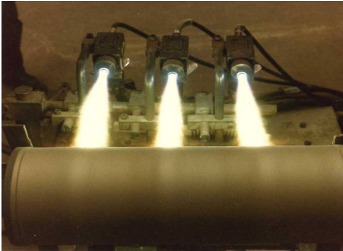
Wallex 50SA applied to a valve stem by three Spraywelder™ Systems
