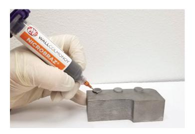
The shelf life of Nicrobraz® Brazing Paste materials is a minimum range of three to nine months (see table). This means that the material will last at least that long and much longer, when properly stored in closed containers. There is no deterioration of the brazing filler metal itself. As long as the material will extrude from the cartridge satisfactorily, it is still usable.
