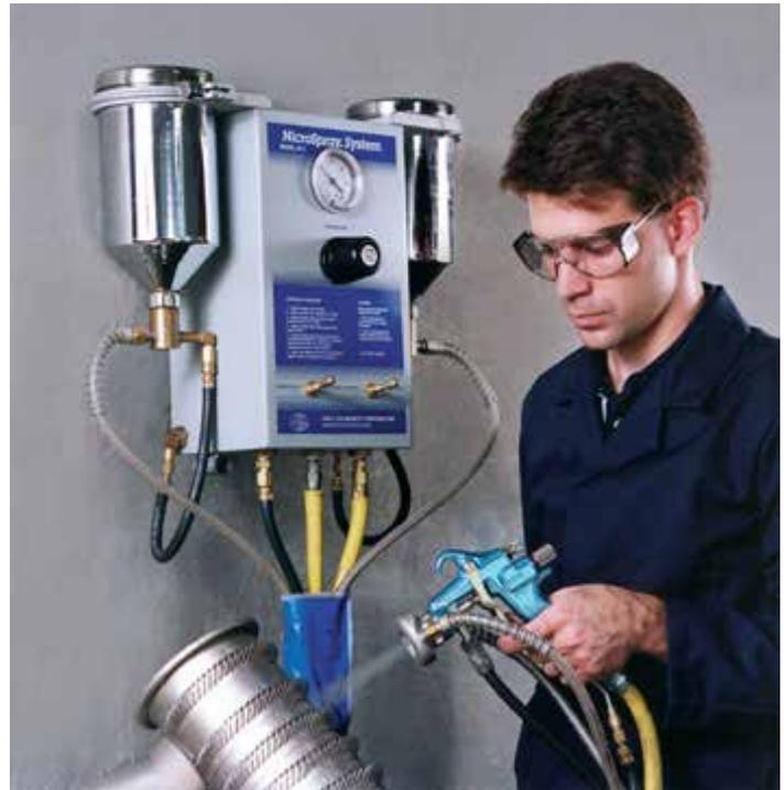
Model N-5 has two powder hoppers. This allows you to operate continuously (switching from one hopper to the other); use both hoppers for higher rates; switch between two different powders; or blend two materials.
