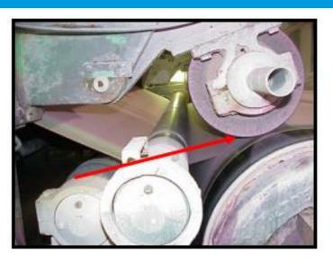
Figure 18. Nip hazard between support rolls and wire.
