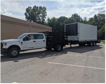
Nanogrid Solutions with 90 sq. Ft of floor space that can serve as Mobile Disaster Command Centers or can be customized to your needs. Many built-in options available such as counter height desks, individual workstations, file cabinets, shelving, pegboard, multiple entrances, air conditioning and export power for telecommunication and broadband equipment. The Nanogrids can be towed on flatbed trailer using a pickup truck.
