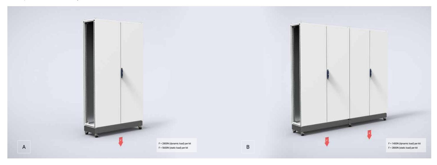
For easy transportation of an (equipped) enclosure, nVent HOFFMAN offers the LCR casters. The casters can be mounted directly on the enclosure's frame or underneath the plinths (PF/PV) with the provided mounting brackets. The use of LCR casters raises the enclosure by 70 mm.
