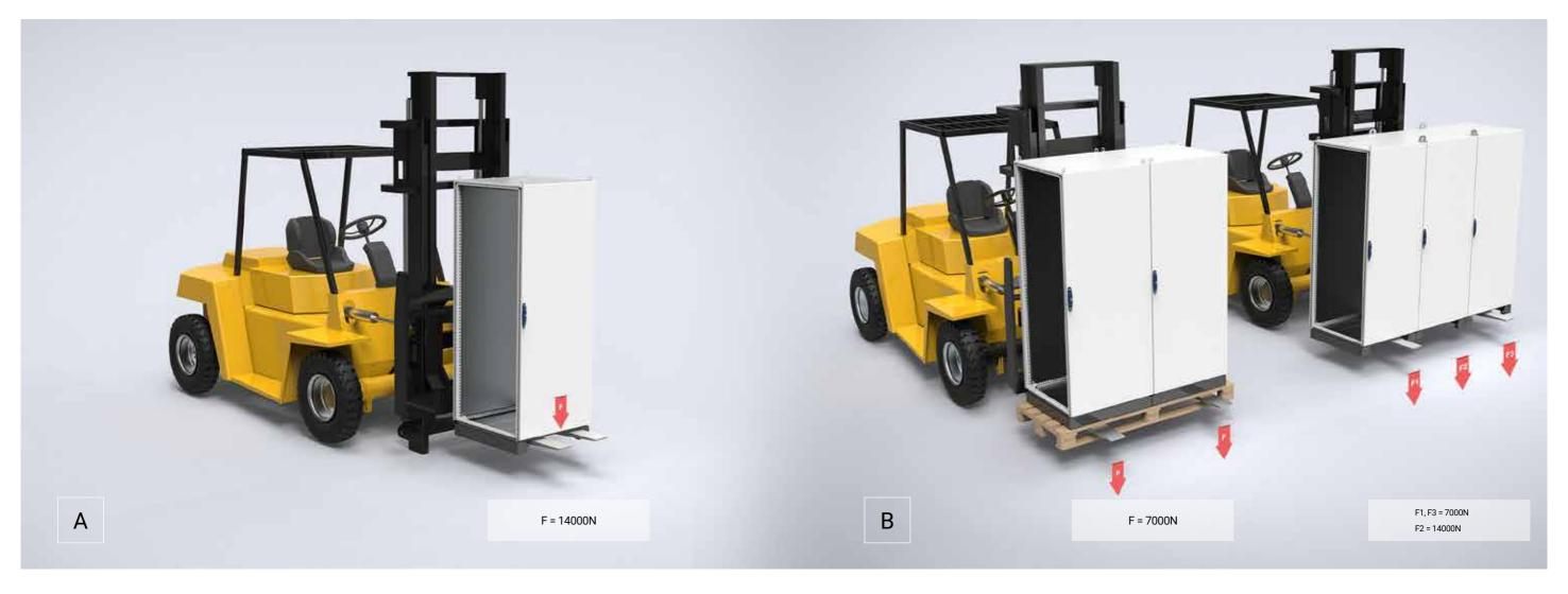
nVent HOFFMAN's floor standing enclosures are suitable for transit by forklift truck either individually or as a bayed solution. In either case it is important that the applicable plinths are fitted to ensure that the forks of the forklift truck can be moved underneath the enclosure(s) in order to safely transport them. For a bayed floor standing enclosure solution, nVent HOFFMAN's combining plinths should be used and fitted between each enclosure for strength and rigidity.
