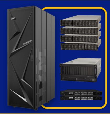
The FlashSystem 9200R is a bundle of products that will be assembled, delivered and configured for the customer.
