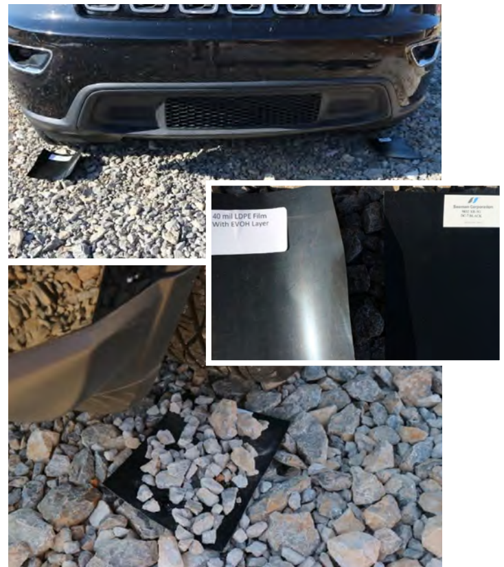
Figure 3. Samples (40-mil LLDPE-EVOH was used for the field test in order to measure a more robust product.) (inset) and Placement (top and bottom) for Field Puncture Simulation
