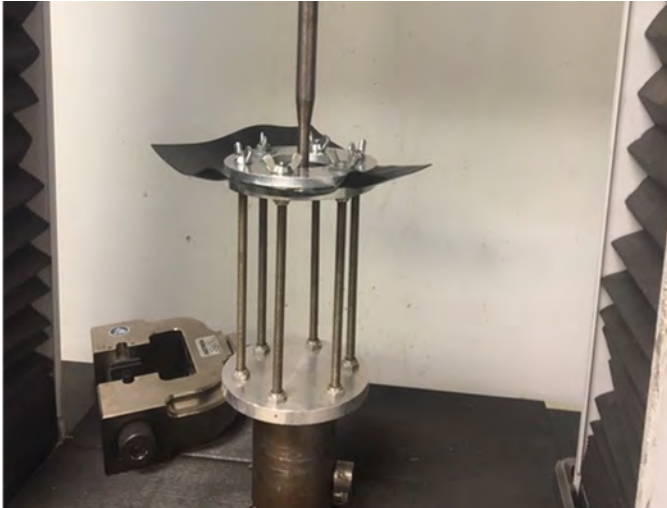
Figure 2. Laboratory Puncture Test Apparatus for ASTM D4833
