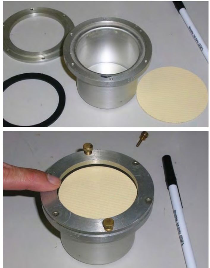
Figure 1. Vapor Transmission Cups for ASTM D814
