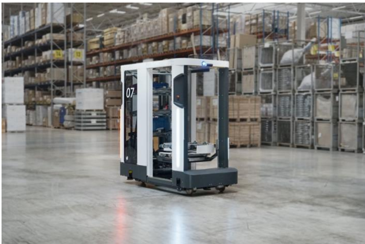
Picture: The robot SOTO enables efficient automated line feeding, for example, in the automotive industry.
