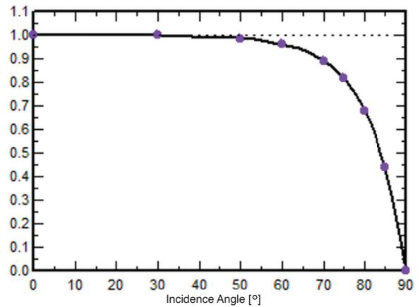
Figure 5: Incidence Angle Modifier.
