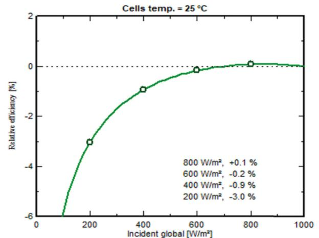
Figure 2: Relative Efficiency With Respect to STC.
