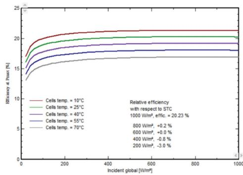
Figure 3: Absolute Efficiency With Respect to Irradiance.
