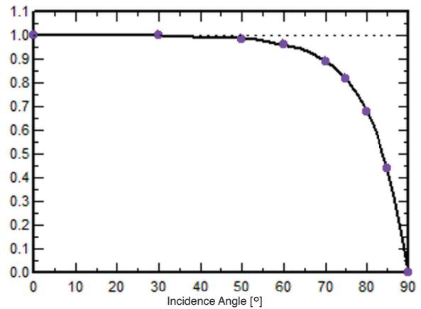
Figure 5: Incidence Angle Modifier.
