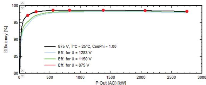
Figure 4: Inverter Efficiency vs. Power Output.
