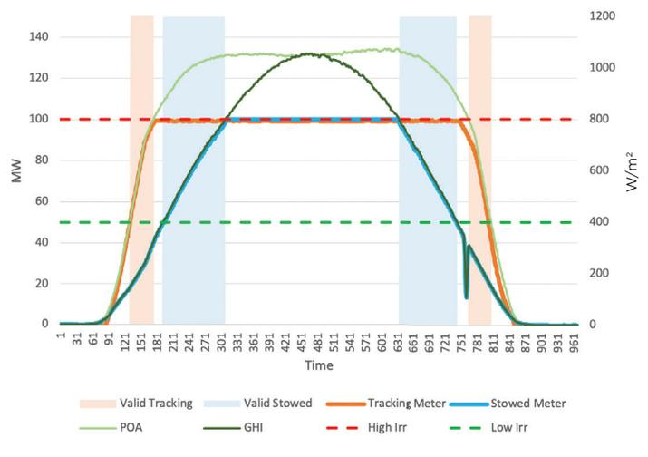
Figure 6: Tracking vs. Stowed.
