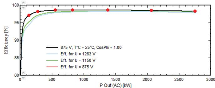
Figure 4: Inverter Efficiency vs. Power Output.
