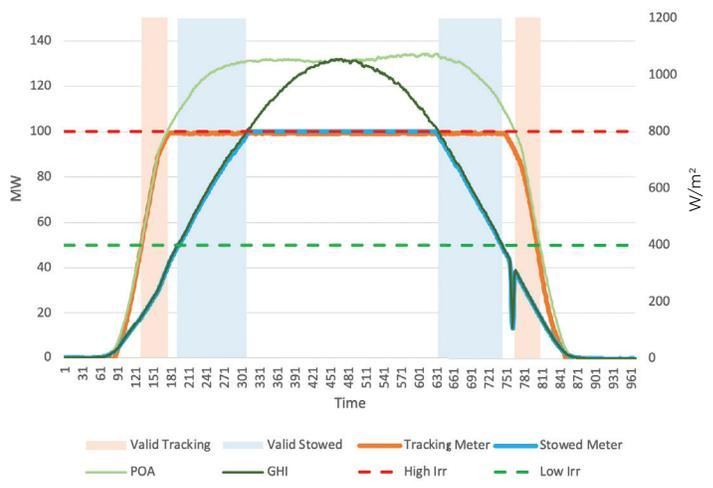
Figure 6: Tracking vs. Stowed.
