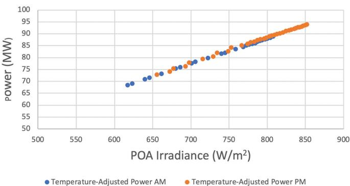
Figure 7: Power Adjusted to 45°C Cell Temperature.
