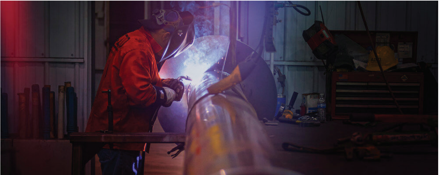
Figure 1: The plasma cutter cuts, copes, notches and splits beams much faster than traditional methods, reducing labor timelines and allowing more projects to be processed through AZCO's prefabrication and modular construction shop.
