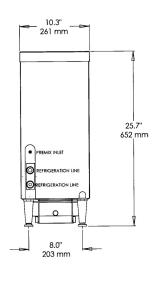
Minimum Wall Clearance Both Sides and Back -6 inches (152 mm)
