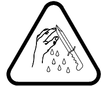
SHARP MACHINE PARTS HAZARD
