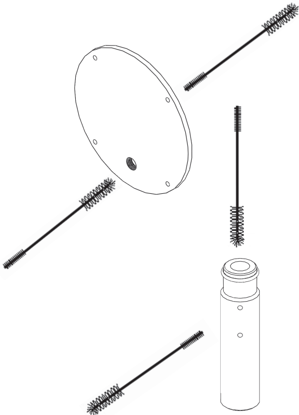
Fig. 15 Clean ALL Holes and Ports with Brushes
