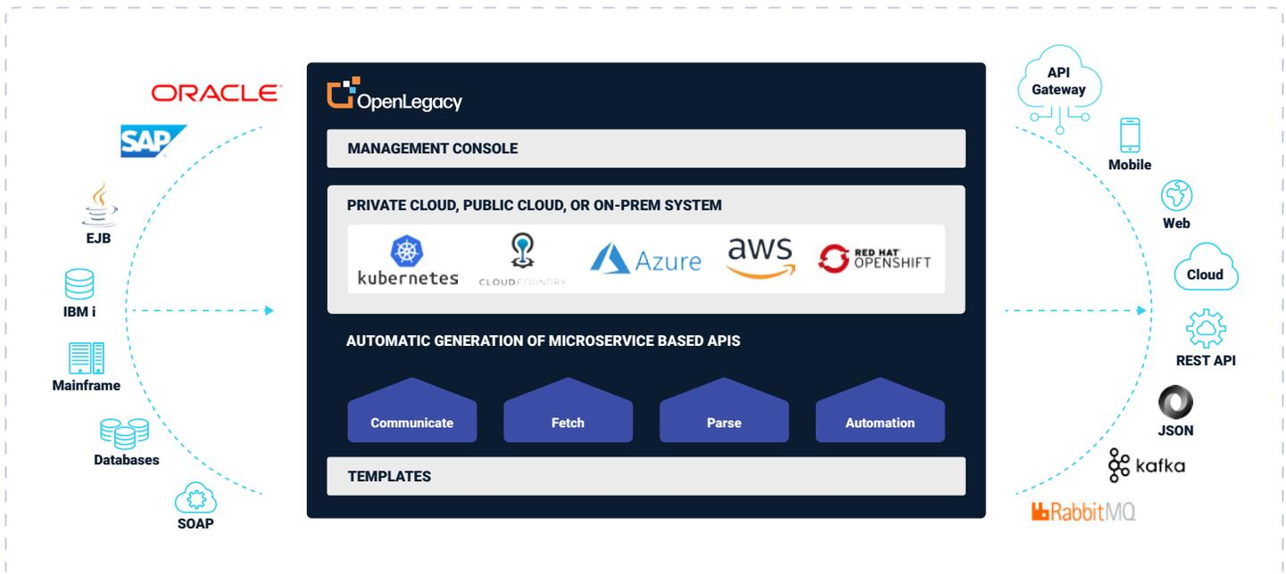
*OpenLegacy platform's overall architecture showing its major functionality, the potential inputs, and how it outputs to a number of different types of systems.*
