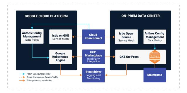
The OpenLegacy Digital-Driven platform enables legacy assets to act as digital ones by automatically generating microservices connected directly to the core systems. Everything connecting to the legacy system is self-contained within the microservice. This self-containment means there is no extra overhead and allows the mesh to focus on the choreography between microservices.
