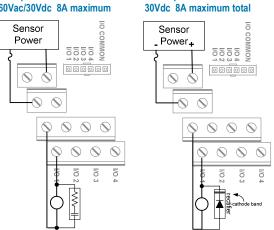
RC or diode snubbers must be used on all inductive loads
