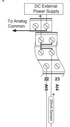
Analog Inputs Wiring Self Powered Devices
