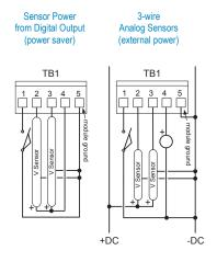
All discrete and analog inputs/ outputs are referenced to the ground terminal (5). This terminal is connected internally to the modules power supply ground.
