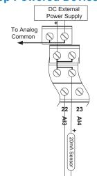
Analog Inputs Wiring Self Powered Devices
