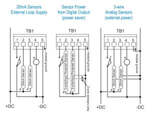
All discrete and analog inputs/ outputs are referenced to the ground terminal (5). This terminal is connected internally to the modules power supply ground.
