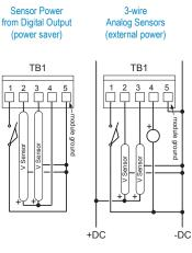
All discrete and analog inputs/ outputs are referenced to the ground terminal (5). This terminal is connected internally to the modules power supply ground.
