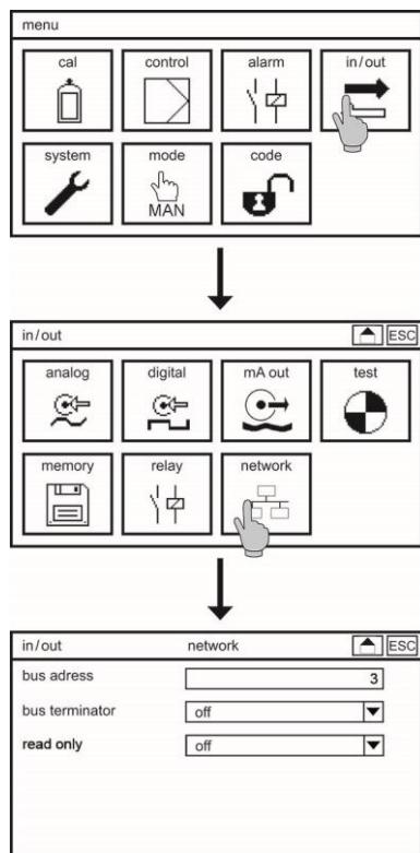
Select the symbol IN/OUT in the main menu and in the submenu, select the symbol NETWORK. Here you can set the following parameters:
