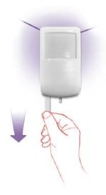
6. Press the left side of the device hard against the wall for 10 seconds until the device is securely attached to the wall. Make sure that the whole of the sticking pad is in contact with the wall.
