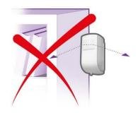
A location that has moving objects near the MDsense. For example, curtains or light fixtures with hanging parts.
