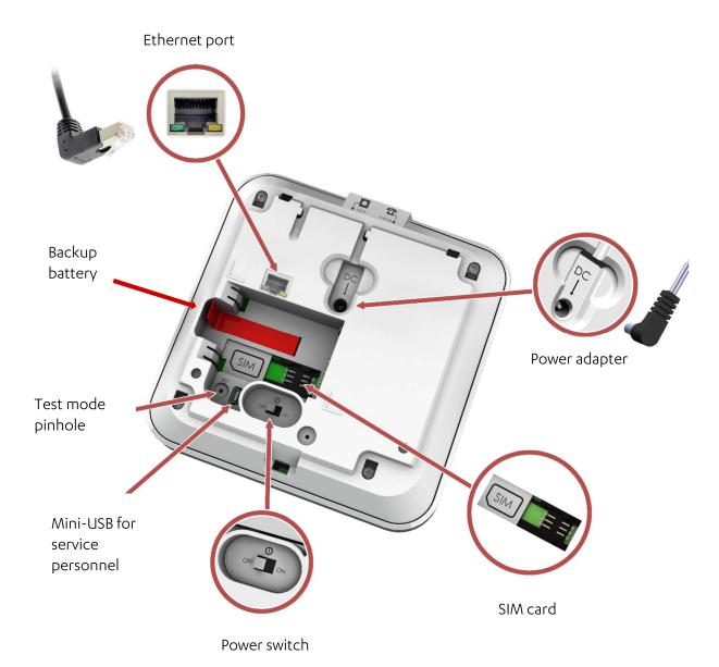
The C7000 has a rechargeable battery as a backup power source. The C7000 communicates with the monitoring station using a cellular network or a standard telephone network Public Switched Telephone Network (PSTN) landline or Ethernet, according to the C7000 version. Cellular and Ethernet communication are supported by Pro, Family, and PERS. PSTN communication is supported by PERS. If there is a communications failure, the C7000 saves messages and sends them when communications are restored.
