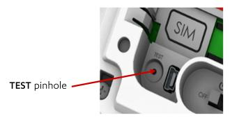
The C7000 LEDs flash and the C7000 beeps three times. The C7000 is restored to factory settings.
