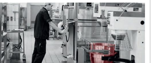
A 100 litres mixer bowl easily weighs in excess of 100 kg, when loaded, and is almost impossible to lift and shift around. An INOX lifter enables you to easily get hold of the bowl and lift it, shift it around, position it at a suitable height, rotate the bowl and pour the contents into a pan or the dough onto the table.
