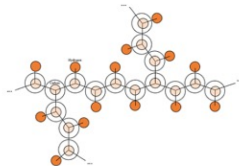
FIGURE 4. Cross-linked Polyethylene (PEX) Molecule
