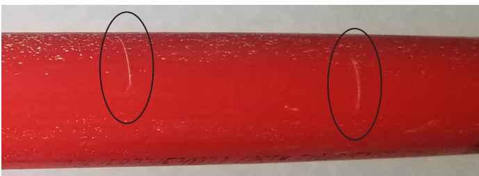
FIGURE 1. PEX failure resulting from a combination of mechanical stress from bending and chlorine induced degradation*
