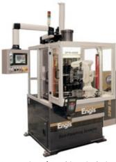
The SPM series of machines is designed to meet the needs of job shops for small to medium size parts. Available in 4, 6, 8 and 10 spindle models, these systems are primarily for bores up to 51mm (2") diameter.
