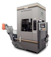
Specialty Custom Machines are designed to meet each customer's specific requirements. For example, in finishing Hammer Forged Rifle Barrels we included a precision reaming station for roughing followed by a series of 8 single-pass honing tools.
