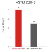
Sustained Pressure Test at 82°C
