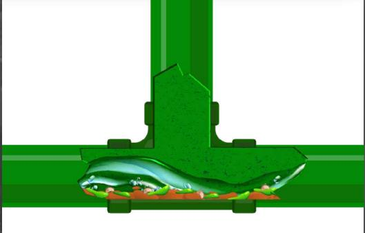
Biofilm is formed over time on surfaces in wet environments, such as pipes used to transfer liquid. It adheres to the inner surface of the pipe, forming a slimy, glue-like substance where bacteria can form and grow. Gradually, biofilm becomes capable of releasing microorganisms and bacteria into the water. This release of bacteria can not only alter the quality of water, but it can also lead to a number of known illnesses.
