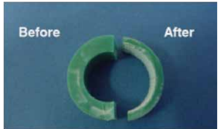
PPR Erosion After 9-1/2 months (at 5ppm Chlorine)
