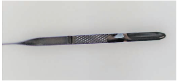
FIGURE 13-14 Hold the dipstick level when reading it.
