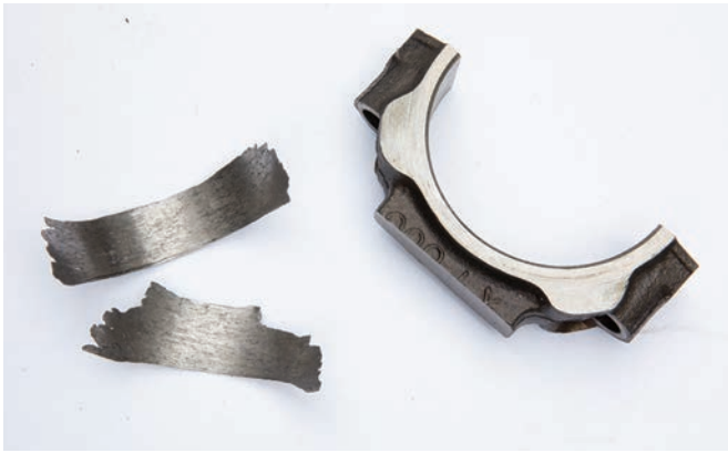
FIGURE 13-11 Parts damaged by lack of lubrication.
