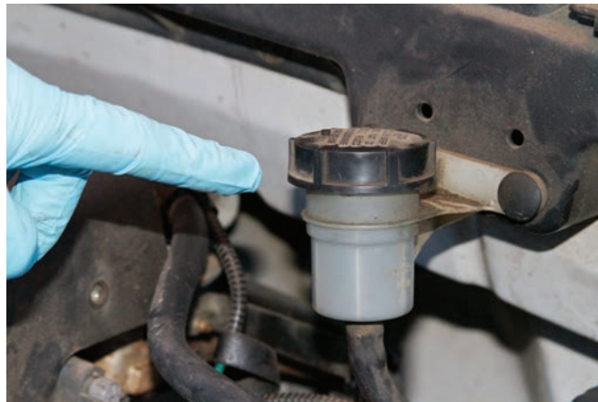
FIGURE 13-21 Some hydraulic clutches use a reservoir separate from the brake master cylinder.
