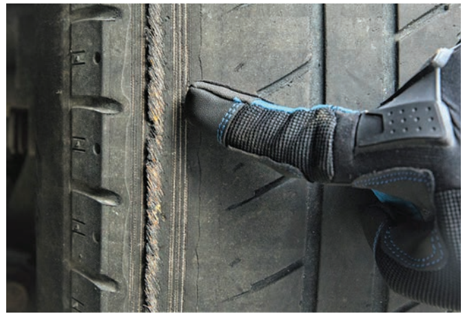
FIGURE 13-46 Because bulges in tires are due to broken belts, often the steel cords stick out of the tread. Be careful not to run your hand across them.
