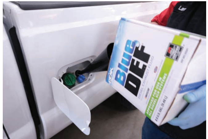
FIGURE 13-28 Adding DEF to the reservoir.
