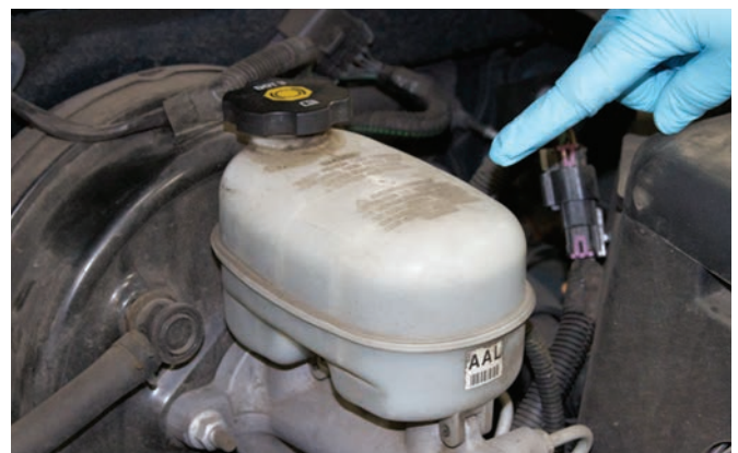
FIGURE 13-20 The brake fluid is stored in a reservoir attached to or near the brake system master cylinder.
