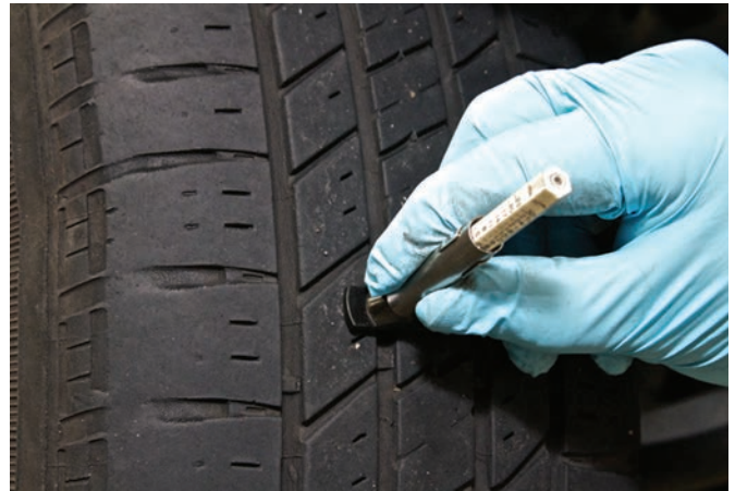
FIGURE 13-45 Tire being checked for wear patterns, damage, and tread depth.
