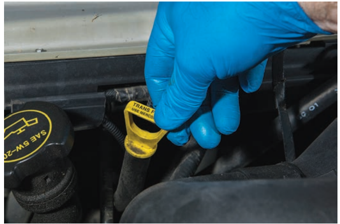
FIGURE 13-24 The transmission dipstick is usually located near the front of the transmission.
