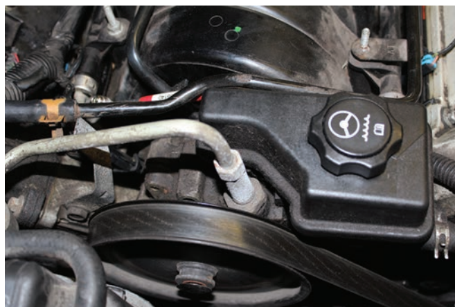
FIGURE 13-21 Some hydraulic clutches use a reservoir separate from the brake master cylinder.
