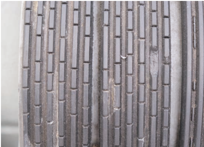
FIGURE 13-31 A serpentine belt with excessive cracks should be replaced.
