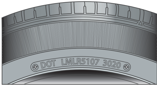
FIGURE 13-47 Four-digit DOT date code showing that this tire was manufactured in the 30th week of 2020.
