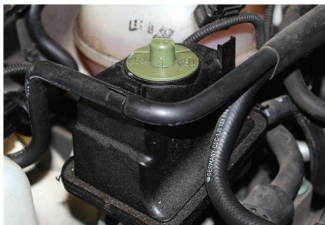
FIGURE 13-22 The power steering fluid reservoir. A. Mounted on the engine-driven hydraulic pump. B. Mounted separately.
