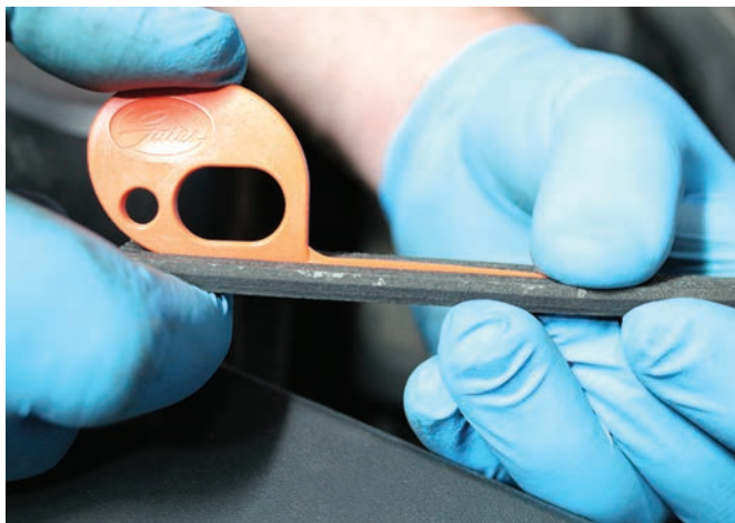
FIGURE 13-36 A serpentine belt wear tool should fit into each groove and still stick up higher than the ridges in the belt.
