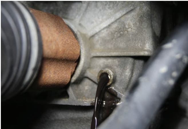
FIGURE 13-27 On transmissions with a fill plug on the side of the transmission, fill until transmission fluid just starts to come out.
