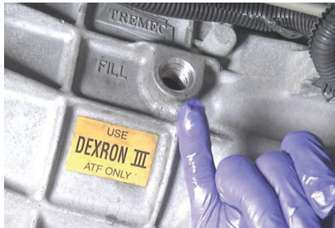
FIGURE 13-48 Checking the transmission fluid level in a manual transmission. (Note that this manual transmission specifies automatic transmission fluid.)
