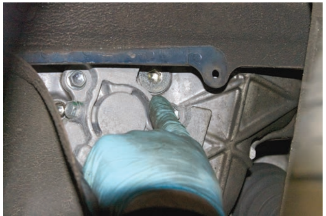
FIGURE 13-25 Some automatic transmissions are checked using a fill plug, or level plug, on the side of the transmission.
