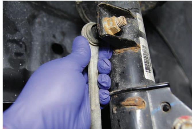
FIGURE 13-51 Torn dust boot and worn joint on this stabilizer link.
