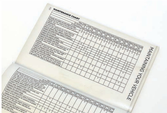
FIGURE 13-17 Service information listing the recommended oil and filter change mileage or time interval.
