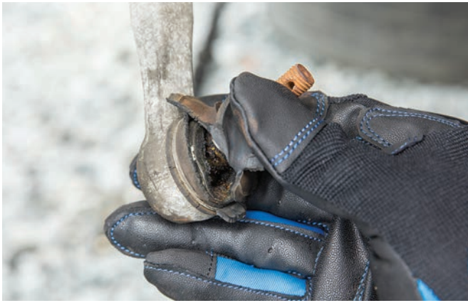
FIGURE 13-49 Extremely worn steering components (tie-rod end) cannot hold the wheels in the correct position (removed for better view).
