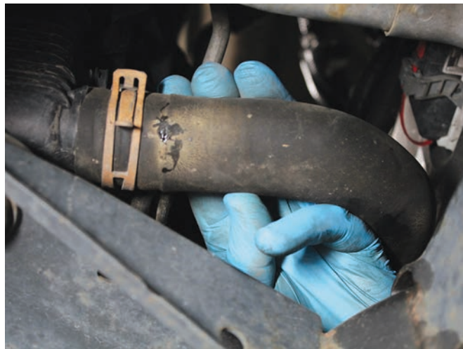
FIGURE 13-53 Lower radiator hoses get neglected and need to be inspected.
