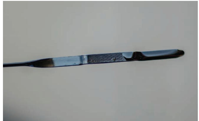
FIGURE 13-15 Flip the dipstick over and compare the reading on both sides. The lowest reading is the most accurate.
