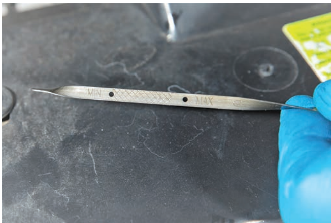
FIGURE 13-13 Oil dipsticks typically are labeled either full and add or min and max .
