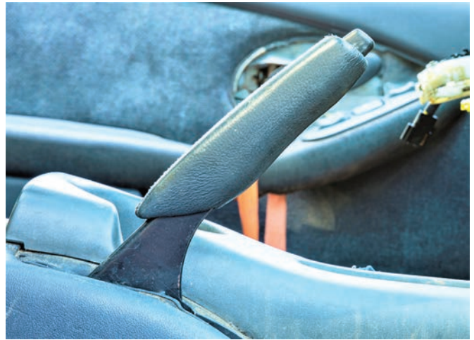
FIGURE 13-7 This parking brake goes too far before it is fully applied, requiring further attention.
