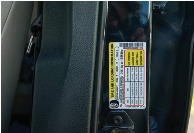
FIGURE 13-42 Typical tire placard located on the door pillar.
