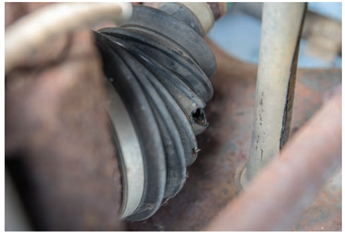
FIGURE 13-52 A torn CV boot found during the inspection.
