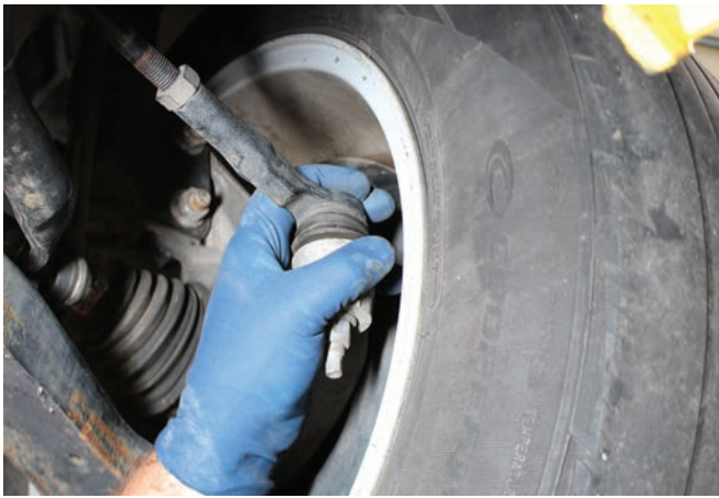
FIGURE 13-50 Wiggle one front wheel left and right while someone is feeling for play in each joint.
