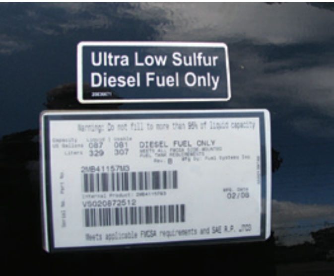
FIGURE 12-11 ULSD fuel is required for all 2007 and later diesel engines equipped with diesel particulate filters. The label on this fuel tank indicates that ULSD is required.
