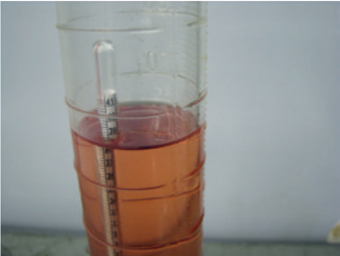
FIGURE 12-21 Reading the API number from the hydrometer.
