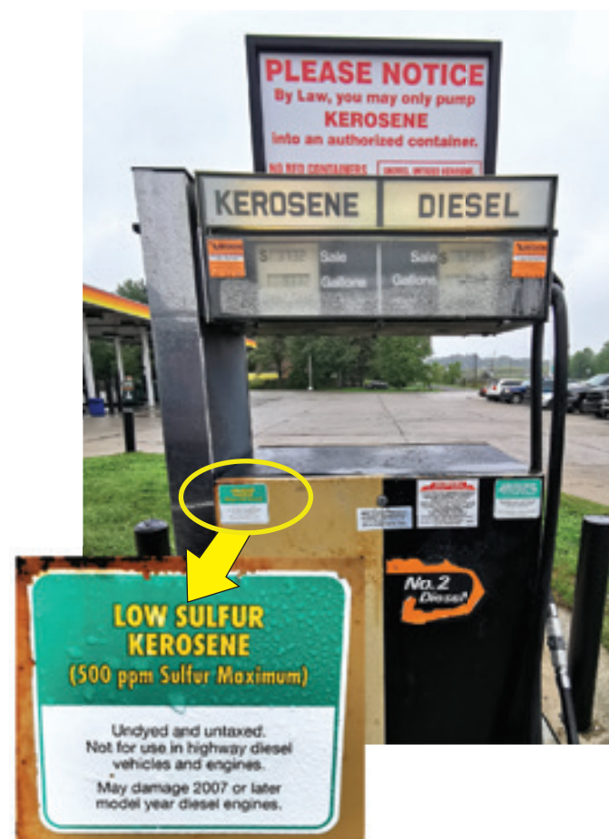
FIGURE 12-2 Kerosene, commonly used as home heating oil and in older, off-road and farming equipment, is a low sulfur content fuel similar to 1-D grade diesel fuel.
