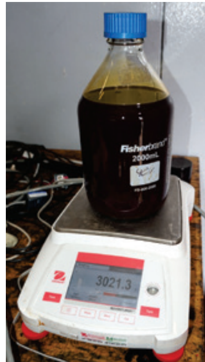
FIGURE 12-6 This jar of fuel capable of burning in modified diesel and jet turbine engines contains liquid smoke derived from pyrolysis of wood chips.
