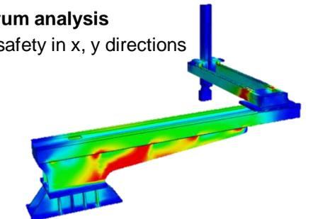
Stress distribution under seismic load
