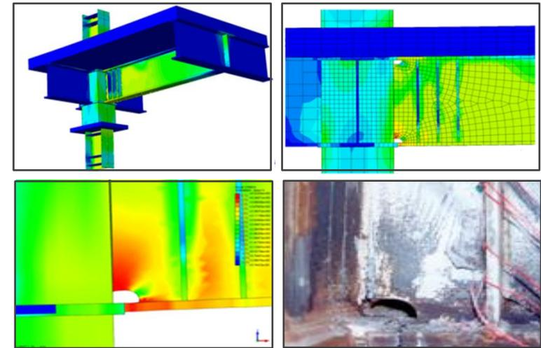
Review energy absorption capacity of the slit damper
