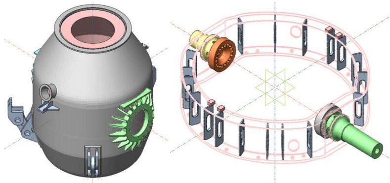
Revolving behavior of furnace:  $-180^{\circ} \sim 180^{\circ}$  around the shaft
