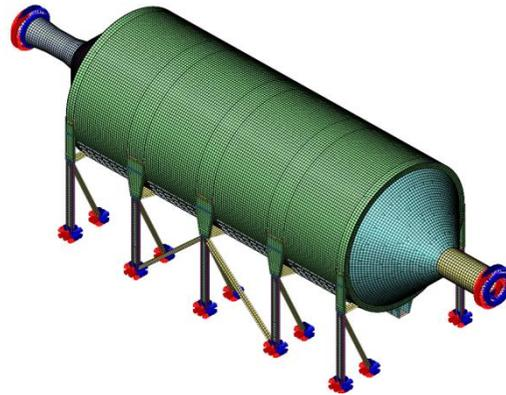
FE model of silo dust collector
