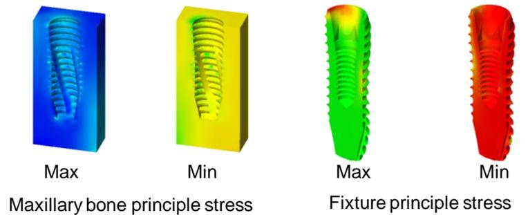
For fatigue analysis result, from 400N, the screw of fixture has a short service life.
