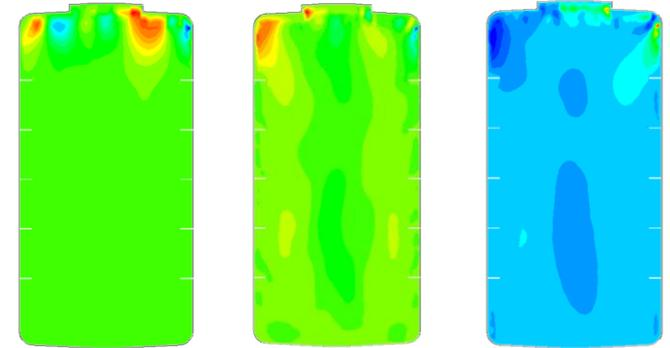
Velocity distribution inside the tank according to time
