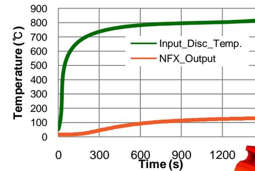
Brake fluid temperature according to time
