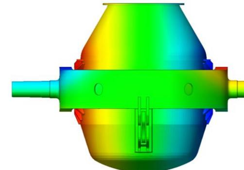
Deformation shape according to heat load
