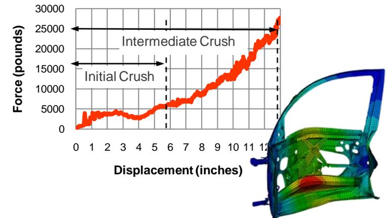
Displacement distribution / force – displacement curve (front door)
