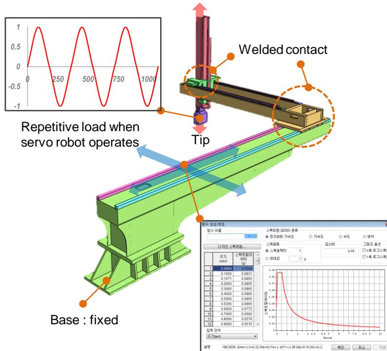
X,Y vibration according to KBC2009 design response spectrum
