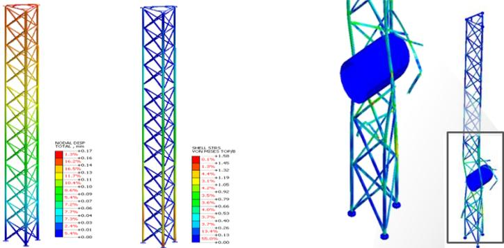
Fracture behavior of antenna tower during the impact
