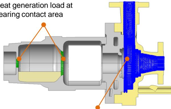
Fluid temperature load inside the housing
