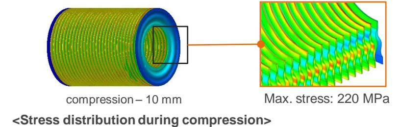
Calculate fatigue life by applying fatigue analysis
