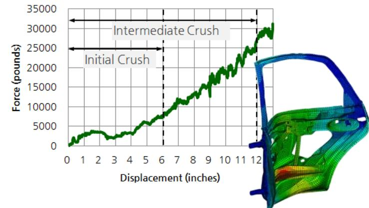
Displacement distribution / force – displacement curve (rear door)
