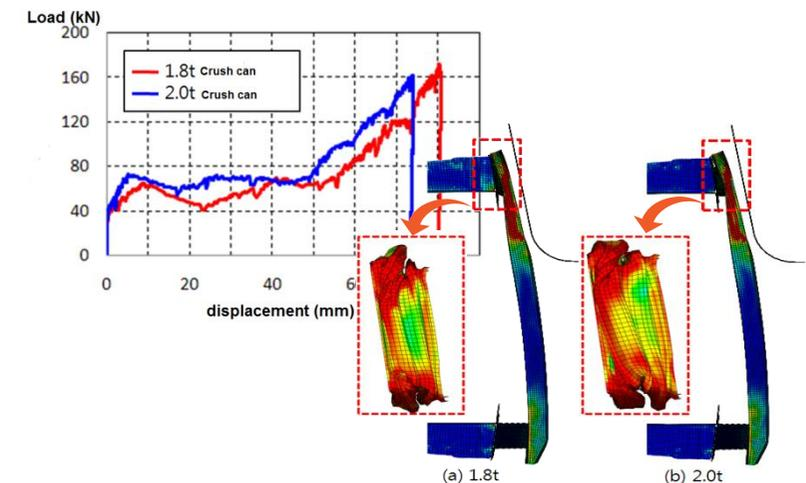
Deformation of the front bumper and crush can
