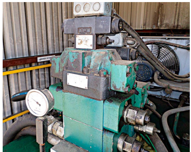
Figure 6. Inspecting hydraulic systems for leaks frequently is an important aspect of system maintenance, but leak reduction can also cut down on contamination ingress.
