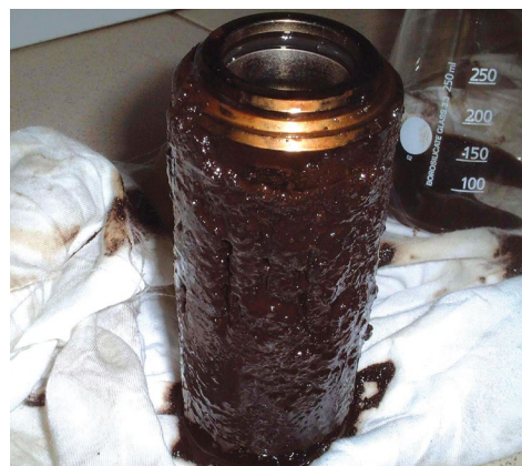
An oil filter from a gas turbine system plugged with sludge. Regular high velocity oil flushing can help keep varnish and sludge under control, but if a filter has already plugged or failed, a high-velocity oil flush may be needed to remove all the debris released into the oil system.
