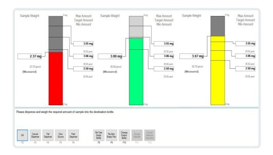
Modified screenshot of the Weighing application to display under/acceptable/over dispenses. (In practice, only the one bar is displayed).
