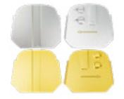
This unique tool contains two ¼ round PCD segments with a single metal-bond segment. Designed for efficient floor preparation, the PCDs aggressively remove floor coatings while the metal-bond segment smooths and refines the scratch pattern. Additionally, the metal-bond segment height is designed to avoid gouging the floor surface with the PCDs.
