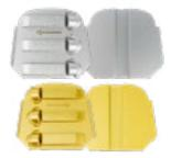
Tackle concrete floor coating, mastic or glue removal with ease using this unique heavy-duty tool. With three large PCDs plus three metal-bond segments, this tool is fast and efficient. The PCDs aggressively attack the floor surface exposing aggregate while the metal-bond segments smooth and refine the scratch pattern. Additionally, the metal-bond segment height is designed to avoid accidental gouging the floor surface with the PCDs.
