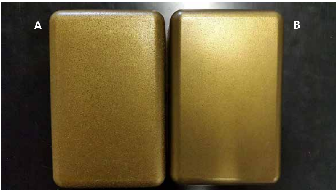
Figure 1 – Parts produced in PE with bronze metallic pigments: a) Uses no enhance and b) uses enhance product at the surface.
