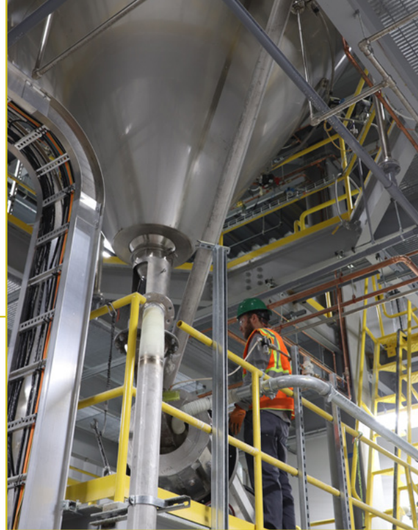
Pictured: Stainless steel drying chamber used to collect the processed powder grains after the heater dries the slurry.
