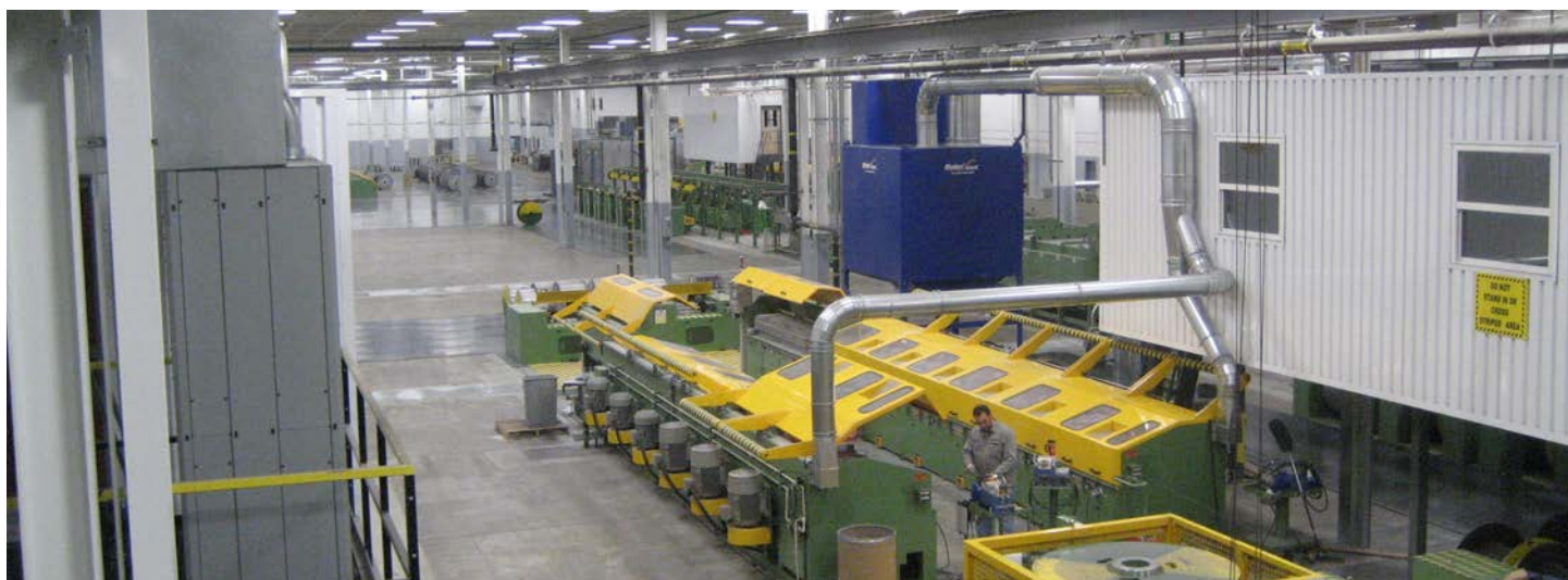
RoboVent unit collecting dust from a weld wire manufacturing facility.
