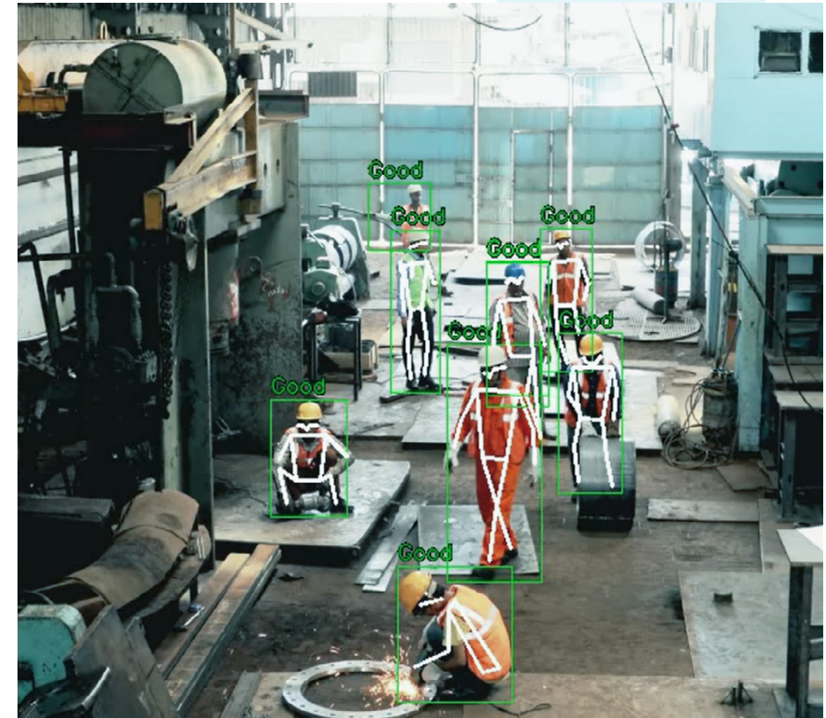
Running multiple neural networks on high-resolution video in tough conditions – detecting protective gear on workers and worker pose estimation for on-site safety monitoring
